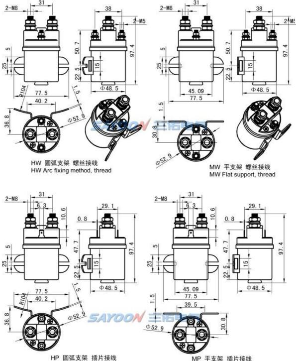
MP 平支架 插片接线 MP Flat support, Spade terminals
